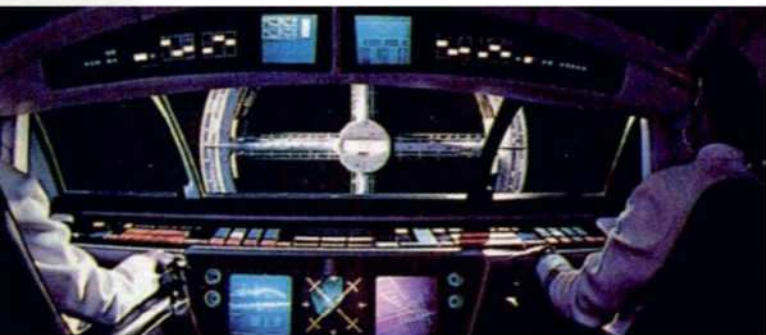
Control deck of Orion is a realistic mockup designed by scientists to simulate controls of 21st-century spacecraft. Pilots must synchronize their course with rotation of the orbiting space station to make a proper landing in the core. Monitors give pilots readouts on proper approach.
